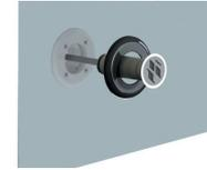
Insert the cable through the inlet and along the pipe.
