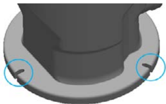
Figure 2 – Floor fixation notches
