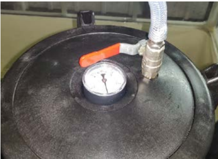
Figure 13 – Quarter-turn valve - recommended pipes in place of the purge screw
